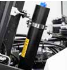
Boom suspension (Nitrogen accumulator)
