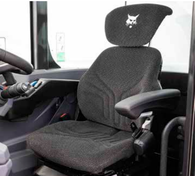
Grammer Maximo air-suspension seat with heating, Dynamic Dumping System (DDS), and a joystick mounted on the suspended armrest
