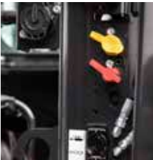
Double-acting rear hydraulic auxiliary outlets and hydraulic trailer brake
